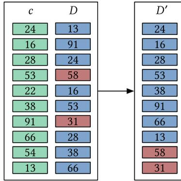
Fig. 6. Reference list re-ranking, where *c* is the *k*-document pre-computed centroid ranking, *D* is the *k*-document SERP generated for the user query, and *D'* is their *k*-document fused result, in this example with *k* = 10 for both. Documents in green are from the centroid list, documents in blue are common to it and the query list, and the documents in red are the ones from *D* that were not in *c*.
