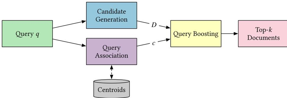
Fig. 5. Modifying the processing pipeline described in Figure 2 to leverage pre-computed query centroids. The user enters a query  $q$ , which is both evaluated against the document collection to create a top- $k$  list  $D$  and also used to search the set of pre-computed query centroids. If a match is found in the cache, then centroid  $c$  and the top- $k$  document list  $D$  are combined by the *query boosting* method, yielding a fused top- $k$  result page.
