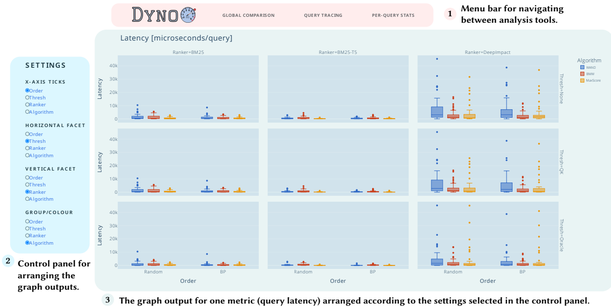
Figure 1: The global comparison page showing the latency profiles of all possible system configurations. Each component of the page is labeled with a short explanation. Note that the global comparison page also plots a number of other metrics such as postings scored .
