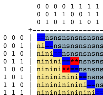
■ Figure 2 All SERP pairs of length k = 3 , and the relationships between them. Red cells indicate non-separability.
